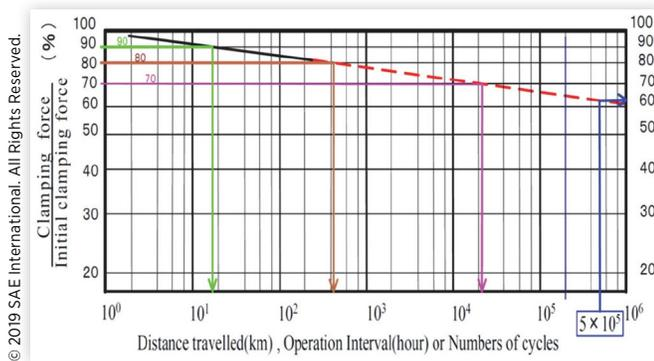
by plotting the measurement results for relatively short-term loosening in the early stages of operation on a log-log graph, and extrapolating the results. When the clamping force residual ratio is 70%, for example, the corresponding value on the horizontal axis obtained with the regression line gives the predicted lifetime. When the distance travelled is 500,000 km, for example, the corresponding value on the vertical axis gives the residual clamping force.
