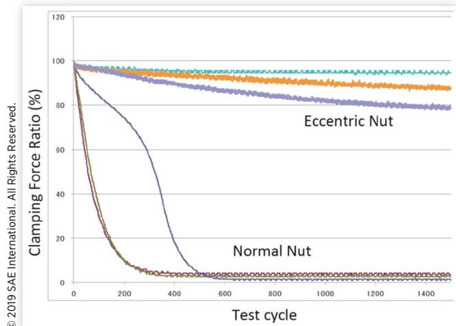
**FIGURE 11** One of the results of loosening test at normal type nut
