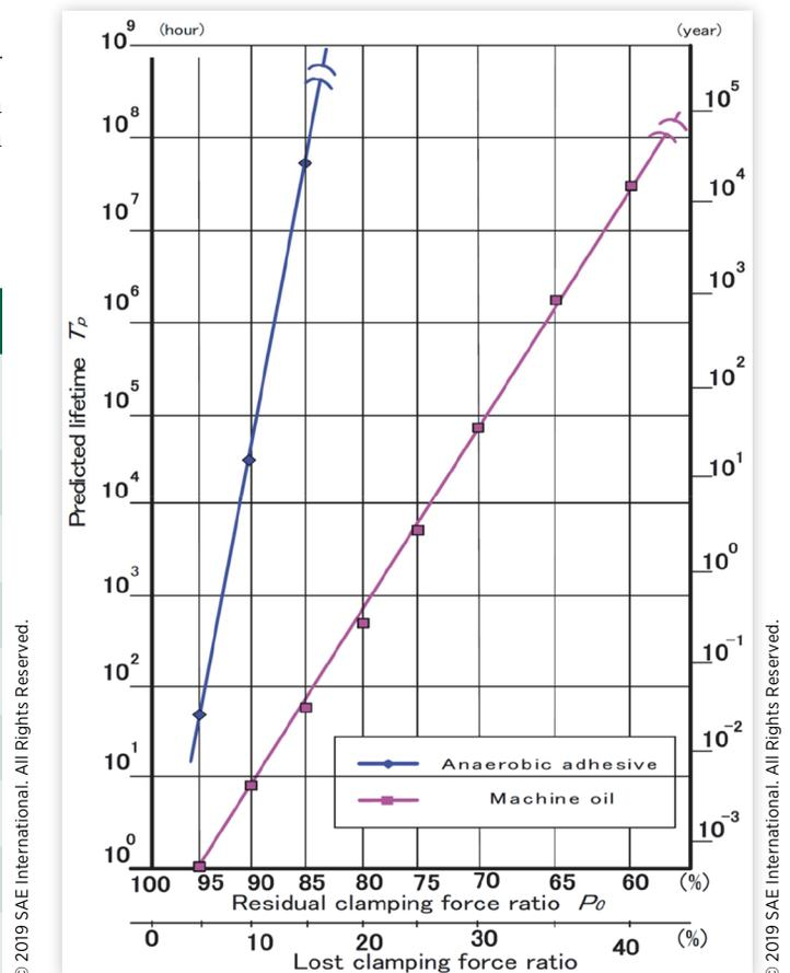
**TABLE 6** Results of lifetime prediction to loosening failure
