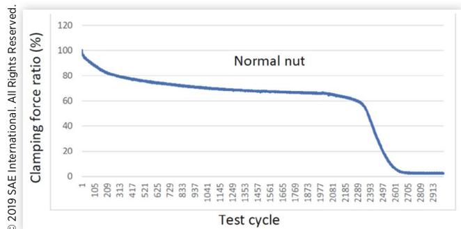
methods is performed using the Junker-style test equipment shown in [Figure 1](#). As shown in [Figure 10](#), the locking effect is evaluated by this loosening test machine for an eccentric nut and a normal nut. Eccentric nuts have good performance in the prevention of loosening. [Figure 11](#) shows the result of a loosening test for a normal nut. A normal nut maintains most of the clamping force for a certain period.
