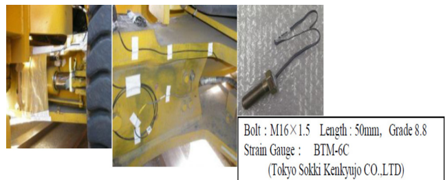
Fig.9 Test Fork-lift Axle and Test Bolt Specification
