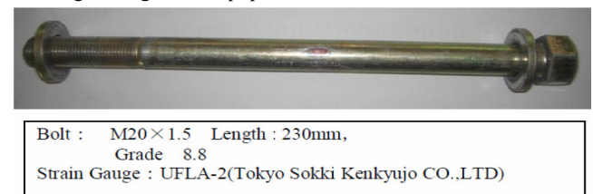
Fig.4 Specifications of a test bolt
