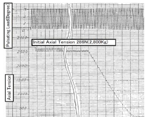
Fig.12: Loosening behavior from testing machine[23]
